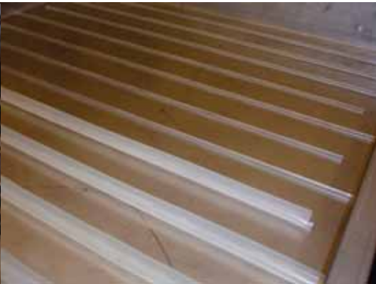
Fig. 3: Photos of the heat storage module with a copper absorber used for the heat transfer.
