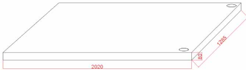
Fig. 6. Principle sketch of heat storage module with two holes used to fill in the salt water mixture.
