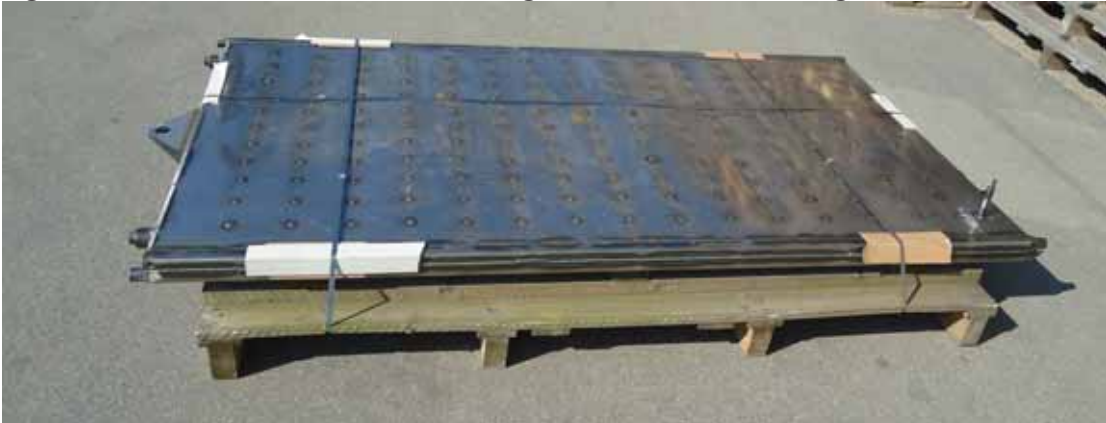
Figure 10: Photo of the third heat storage module with two holes at the left hand side of the module used to fill in the salt water mixture.
