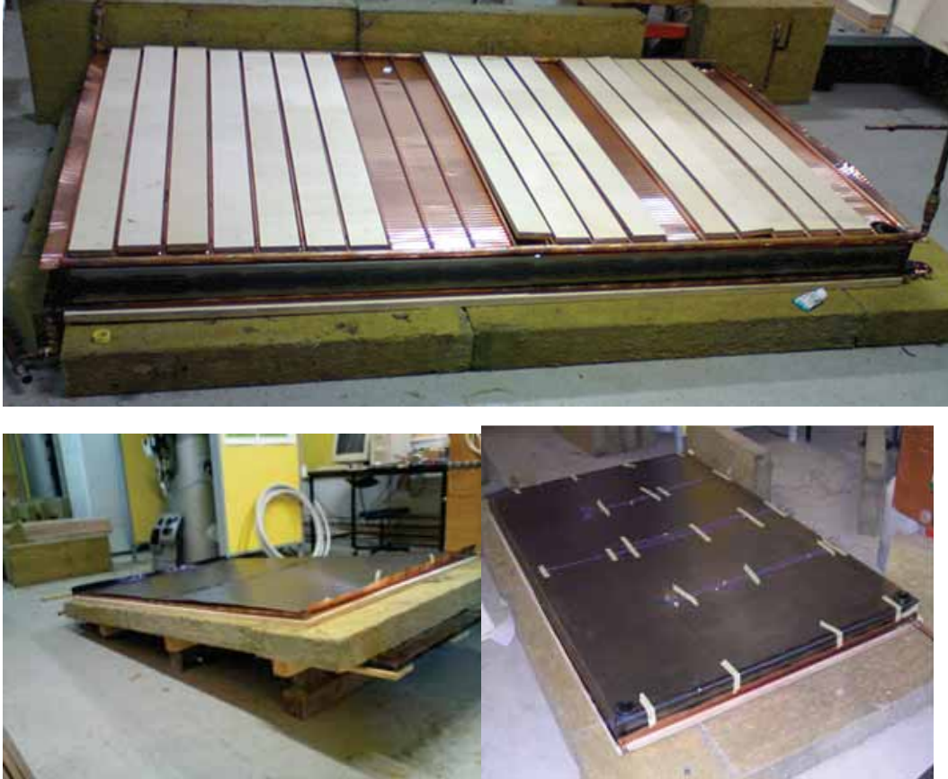
Figure 5: Photos of the first heat storage module.
