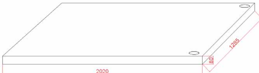
Fig. 1: Principle sketch of heat storage module with two holes used to fill in the salt water mixture.
