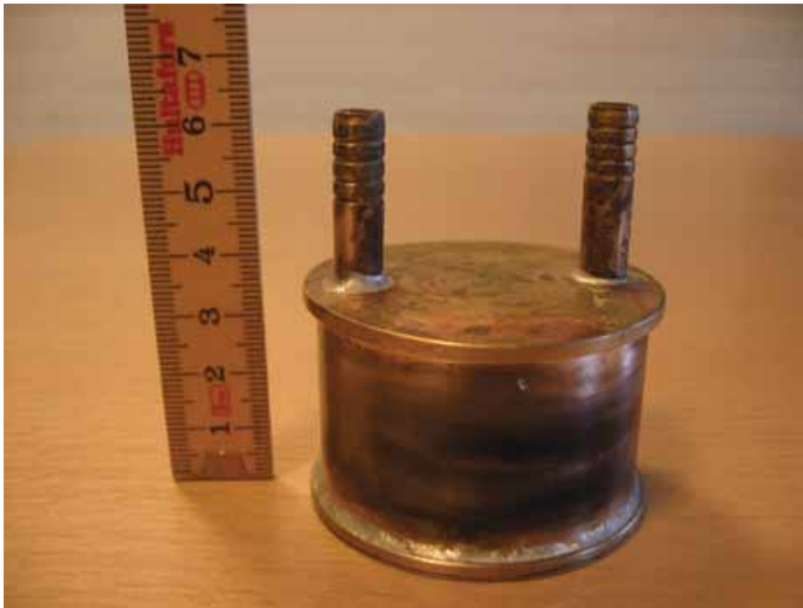
Figure 11: Brass tank with CO 2 used for starting the solidification.
