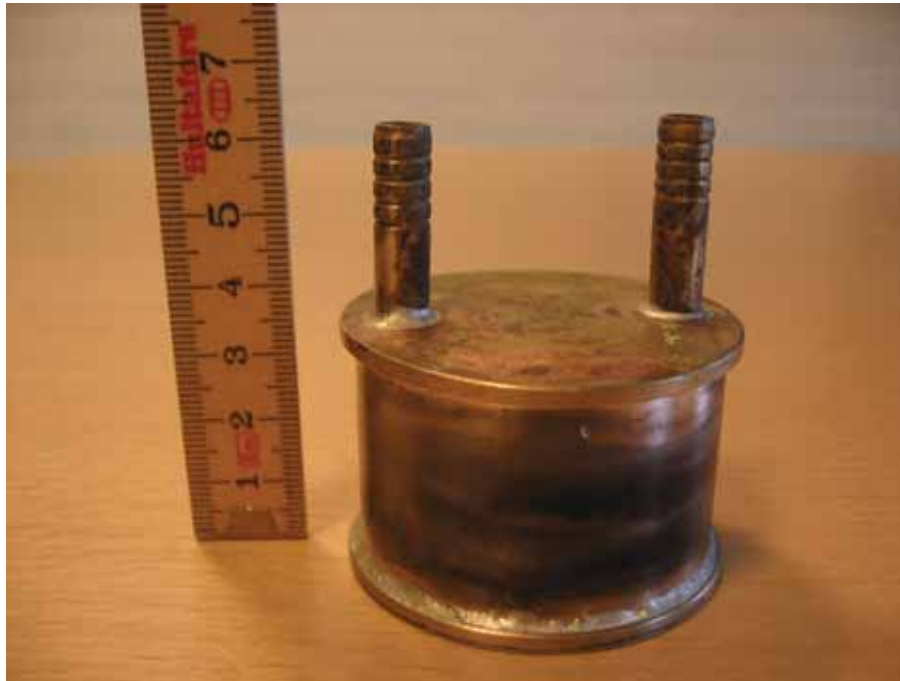
Fig. 9. Brass tank with CO 2 used for starting the solidification.
