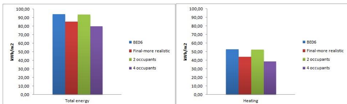
Figure 2: Sensitivity analysis for occupancy. Total energy consumption (a). Space heating demand (b).
