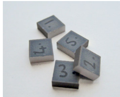
Figure 18: Tiles of piezoelectric material are glued together to build up the glued thickness mode PT.
