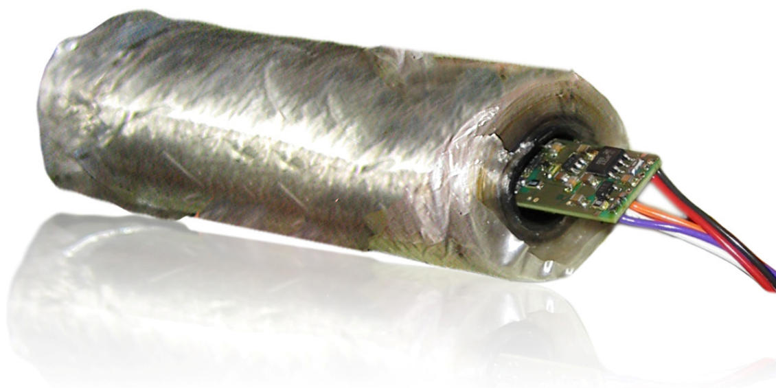
Figure 53: In process of slide the driver into the DEAP actuator.
