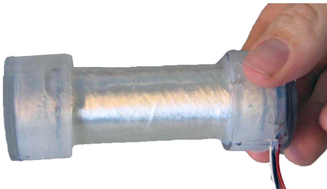
Figure 54: World's first low voltage DEAP actuator
