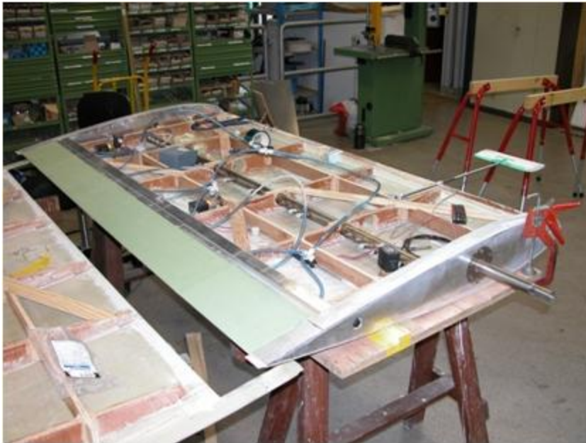
airfoil section + flap during instrumentation
