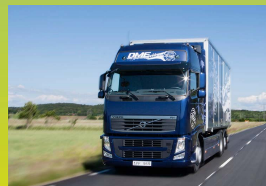
DME powered diesel truck from Volvo
