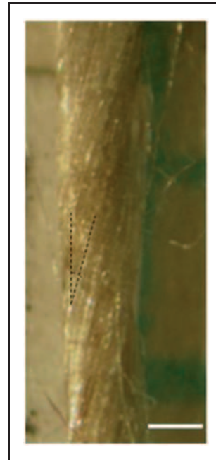
Figure 2. Optical microscope image of the flax yarn (scale bar is 250 \mu\text{m} ).
