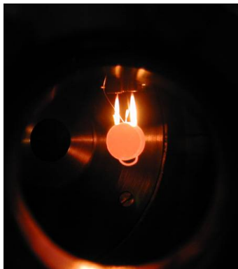
Figure 2.2: Photograph of a Pt(111) sample while heating. Note that this sample is 11 mm in diameter in whereas all samples studied in this thesis are 5 mm in diameter. Photograph taken by Nana Schumacher.
