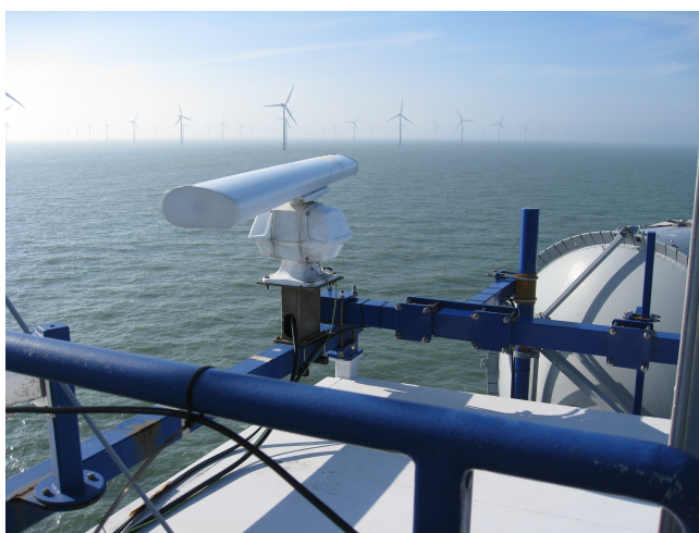
(b) Another LAWR is installed at the Horns Rev 1 wind farm for the needs of a separate experiment.
