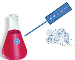
**FIGURE 31 SCHEMATIC EXAMPLE OF AN ANALYTICAL SET-UP FOR SUBSURFACE LASER SCATTERING. LASER LIGHT IS FOCUSED ONTO A SAMPLE AND RESULTS IN A HALO ON THE SAMPLE SURFACE DUE TO SUB-SURFACE PARTICLE SCATTERING. A PHOTO OF THE HALO IS USED FOR DATA ANALYSIS.**
