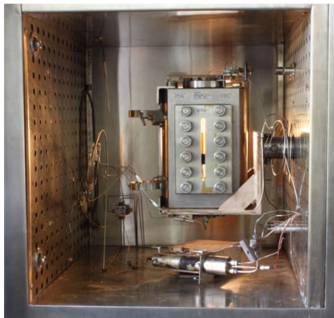
Figure 3. Picture of the DBR JEFRI PVT cell. This is high pressure equipment for phase behavior measurements at various temperatures and pressures. The surrounding steel is the inside of the temperature controlled forced air oven. The cell is monitored on a rocking mechanism suitable for mixing the systems inside the glass chamber. In the middle the glass window is seen which allows visual observations.
