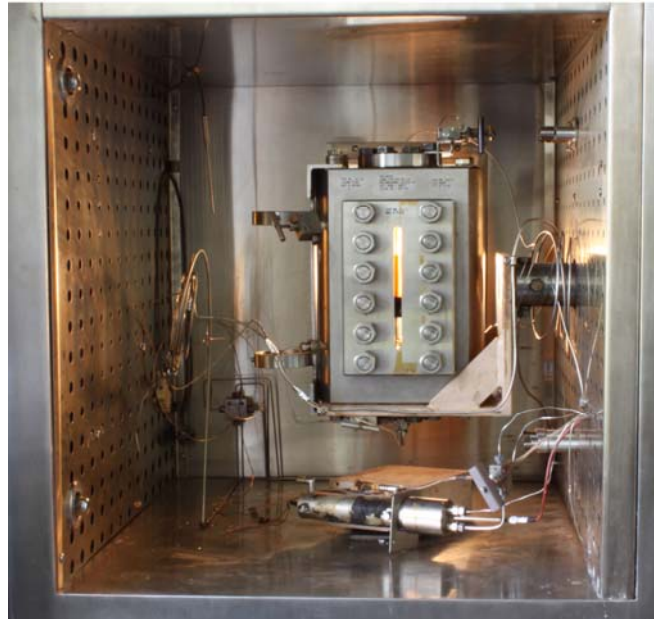
Figure 2. Picture of the DBR JEFRI PVT cell -high pressure equipment for phase behavior measurements at elevated temperatures and pressures. The surrounding steel is the inside of the temperature controlled forced air oven. The cell is mounted on a rocking mechanism suitable for mixing the systems inside the glass chamber. The glass window allows visual observations.
