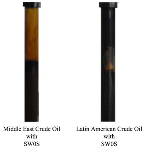
Figure 12. Picture of the formation of a ‘gel’ phase occurring from hand shaking crude oil and brine solution together. This form is stable as long as the glass tubes are at room temperature and atmospheric pressure. The formed phase is sticky and jelly-like. It is immobile, even though it is not completely solid.
