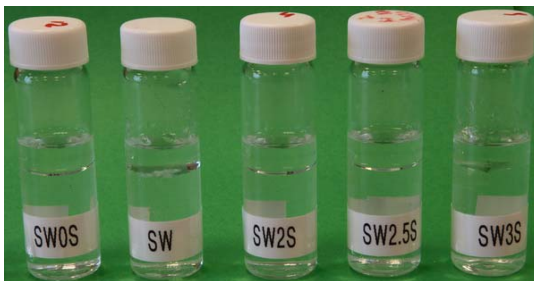
Figure 6. Heptane and different brine solutions after stirring them @ 1000 rpm for 15 mins at room temperature. The sample bottles are filled with heptane and brine solution and have been equilibrated for 1-2 hrs. These tests at ambient conditions were performed to see whether unusual phase behavior or discoloration of the heptane was solely due to the composition of the brine solutions.
