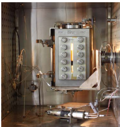
Figure 3. Picture of the DBR JEFRI PVT cell. This is high pressure equipment for phase behavior measurements at various temperatures and pressures. The surrounding steel is the inside of the temperature controlled forced air oven. The cell is monitored on a rocking mechanism suitable for mixing the systems inside the sample chamber. The glass window in the middle allows visual observations.
