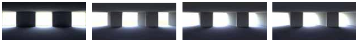
Figure 6 Renderings of the daylight distribution in an east-facing office for various façade angles
