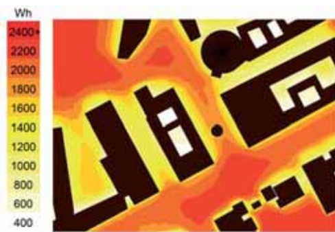
Illustration: Simulation of direct and diffuse solar radiation on Axel Torv, Copenhagen (Wh, daily averages).
