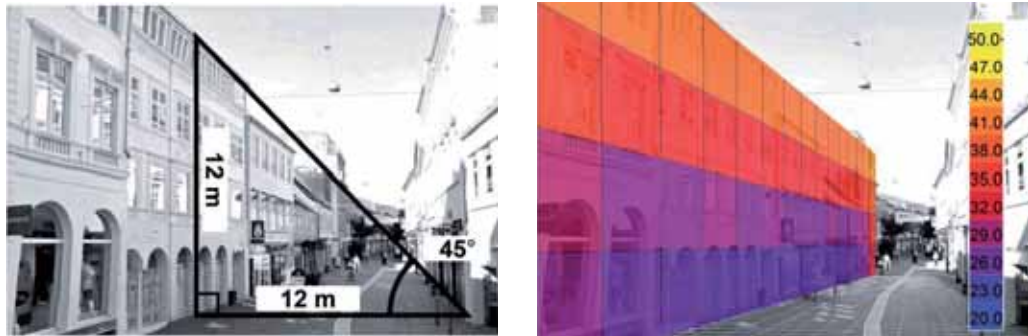
Figure 29: The Vertical Sky Component analysed in Vestergade, Odense city centre. VSC is a measure of the amount of daylight incident on a vertical plane. For a standard overcast sky, the maximum value is 50% (since the point is on a vertical plane, clearly only half the hemisphere can contribute).
