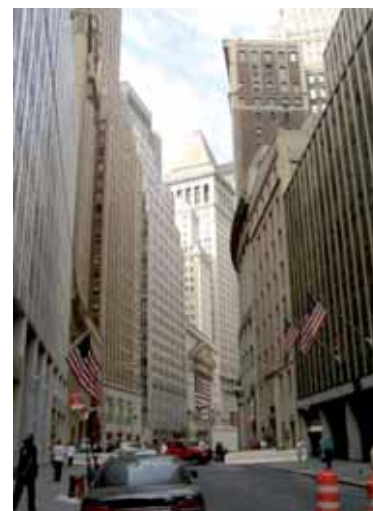
Figure 63: Wall Street Canyon. Façade reflectance approximately equal to 45–55%.
