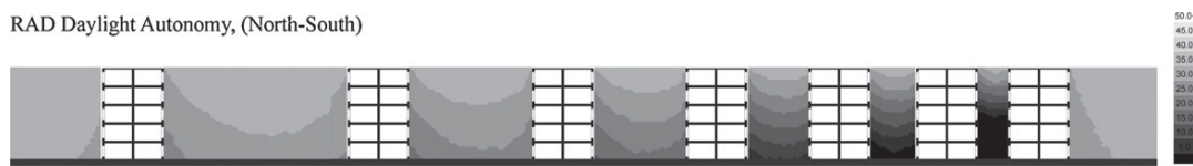
Fig. 6. Annual illuminance >500 lx in street canyon. Performed in RADIANCE/DAYSIM (working hours 08–17, contour range 85–95% in steps of 1%). Weather data, Copenhagen (*epw).
