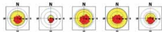
Figure 8: SITE: Solar roses, Copenhagen. From left to right: average hourly radiation on vertical (red) and horizontal (yellow) surfaces, - yearly, winter, spring, summer and autumn averages. Range 0-300wh/m 2 .
