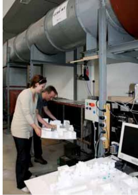
Photo: Students test the wind environment of an urban design at DTU Byg's wind tunnel.
