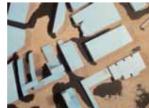
Photo: Erosion testing of urban environment in the wind tunnel (Axel-square Copenhagen).
