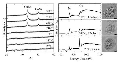
Fig. 1: In-situ XRD and TEM investigation of the synthesis of a CuNi catalyst out of their nitrate salts. The XRD peaks the show formation of CuNi alloy while the EELS spectra show the reduction of the CuO to Cu as the Cu onset peak becomes weaker. The bright field images show the nanoparticle formation (scale bars are 100nm).
