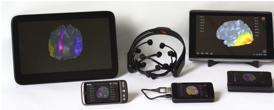
Figure 1: The Smartphone Brain Scanner running on a Linux-based EXOPC tablet (top left), the Emotiv neuroheadset, Android-based Acer tablet (top right), Android-based HTC smartphone (bottom left), Maemo-based N900 smartphone (middle), and a MeeGo-based N950 smartphone (bottom right).
