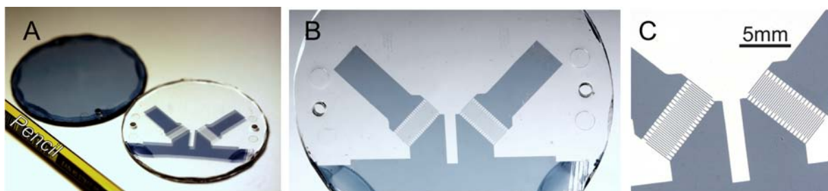
Figure S2. Photographs of PEDOT films on a COC substrate patterned by stamping with an agarose stamp soaked in a solution of 1.5wt% NaOCl and 0.1 vol% Triton-X100 for 4 mins, followed by washing. Pictures A)-C) taken at increasing magnification. A pencil is included for scale in (A).
