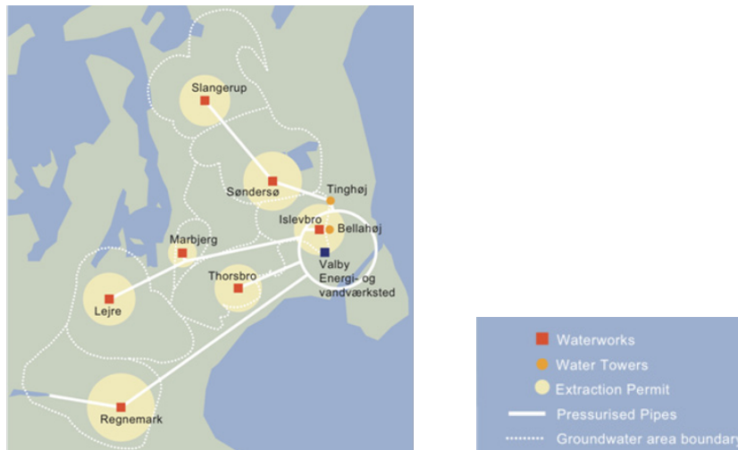
Figure 7. The nodal points of the water supply system in the area around Copenhagen (Courtesy of København Energi A/S)
