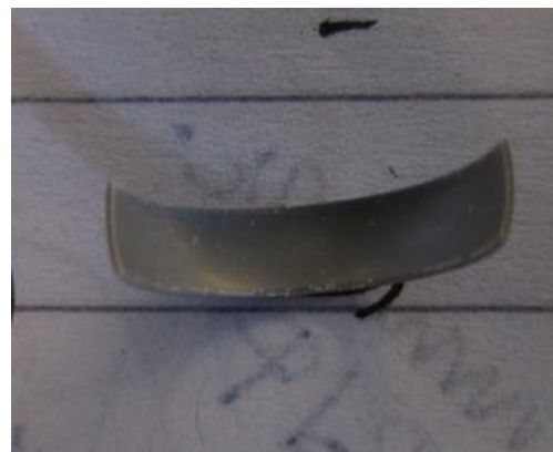
Fig. 9: Image of distortion of bi-layered system after the entire sintering experiment
