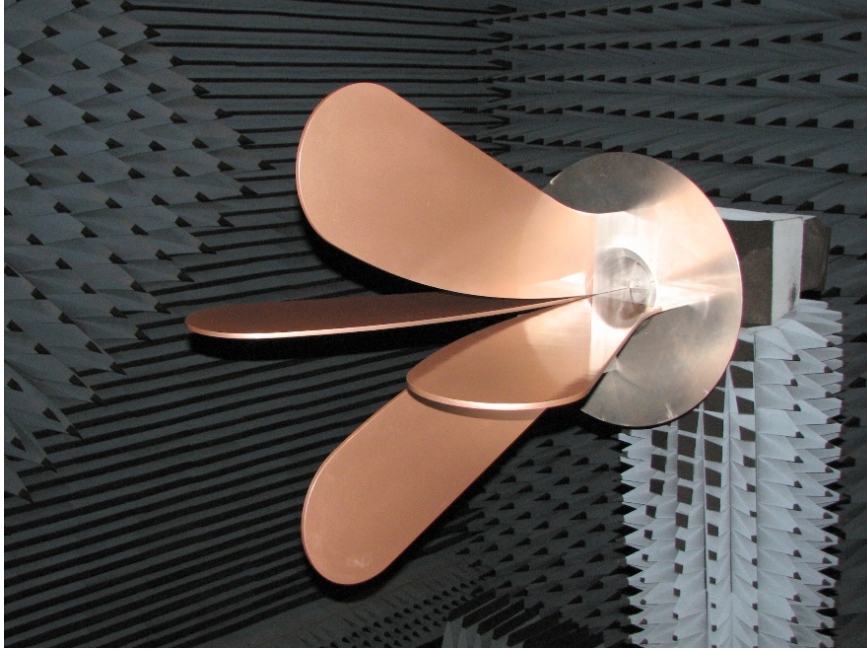
Fig. 20. Manufactured 0.4-1.2 GHz probe during pattern measurements.
