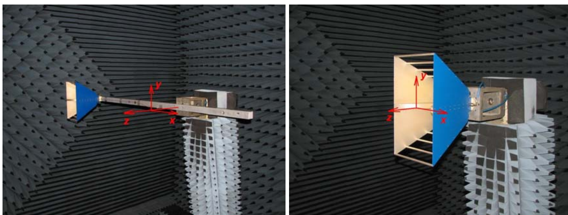
Fig. 27. Offset-mounted (AUT1) and center-mounted (AUT2) SH400 horn used as test object and the measurement coordinate system.
