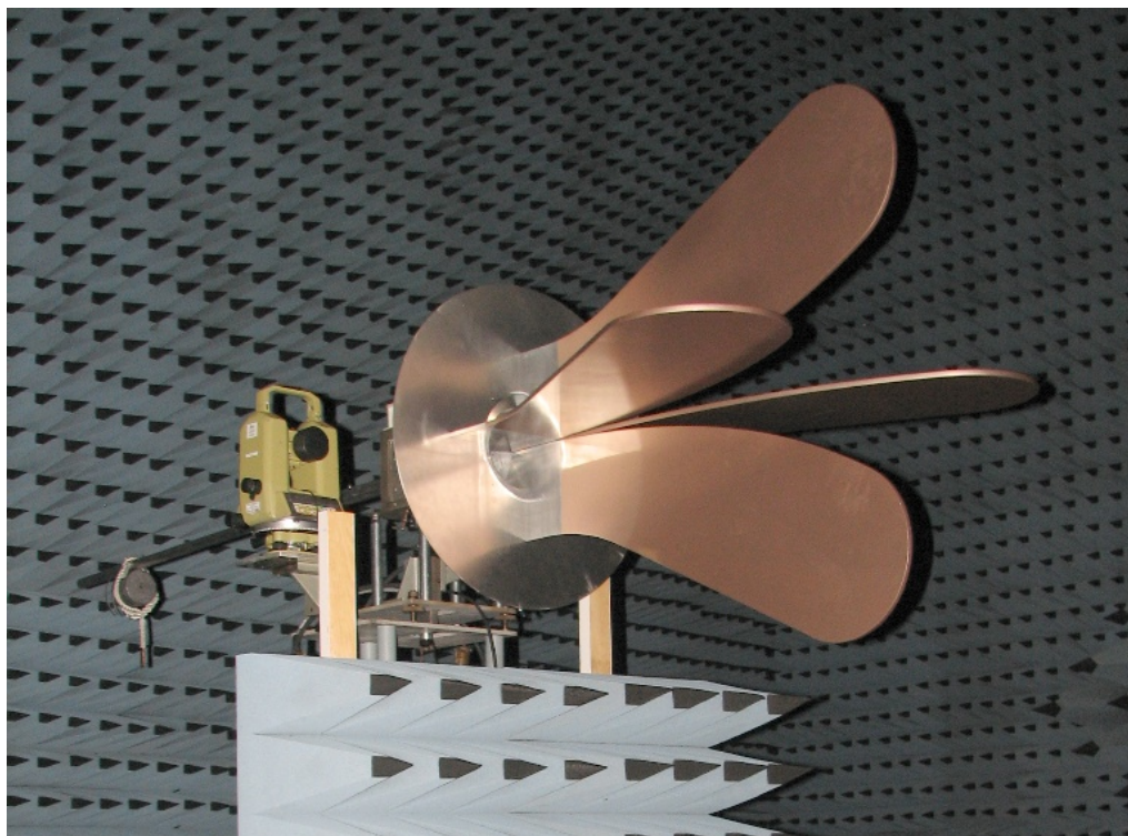
Fig. 2. The 0.4-1.2 GHz probe on the probe tower.
