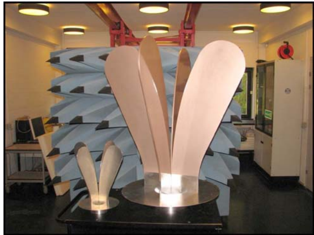
Figure 2 - The manufactured 1-3 GHz and 0.4-1.2 GHz dual-polarized probes.
