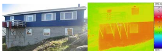
Figure 14: A comparison between a picture of the west façade of the house and the thermographic picture of the west façade
