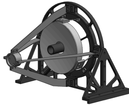
Figure 2. A rendering of the opto-mechanics of the UFFO Pathfinder slewing mirror telescope (SMT).
