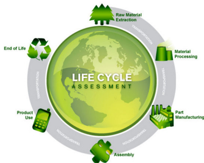
Fig 2.1. A Life-cycle assessment covering all stages in a life cycle from 1) Extraction of raw materials over 2) Manufacturing of a product or system by material processing, manufacturing and assembling to 3) Use phase and finally the 4) End of life treatment.
