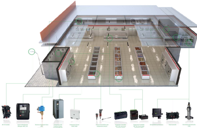
Figure 1.2: Picture of a supermarket refrigeration system including the controller hardware
