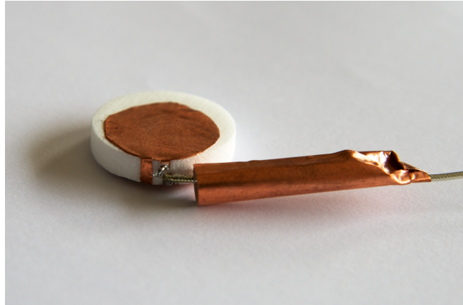
Figure 2: Photo of the constructed antenna prototype.
