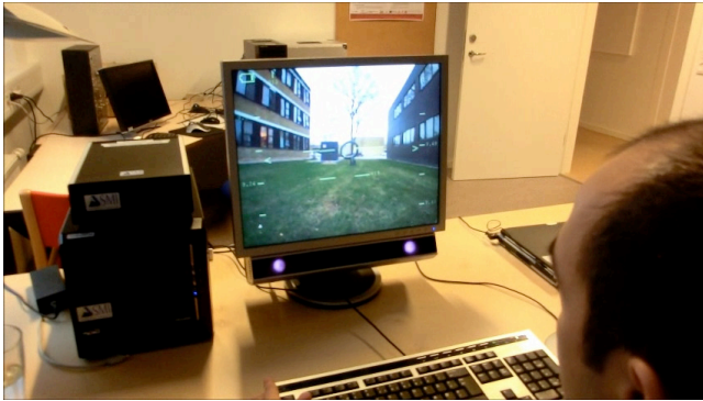
Figure 2. Control room. The point of regard on a video stream is used to control the drone. The eye tracker is positioned below the system display.
