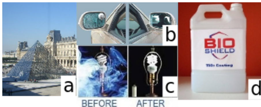
Figure 1.1: Example applications of \text{TiO}_2 photocatalytic properties: a) self-cleansing coating on Louvre pyramid, b) anti-fogging mirrors, c) air purifying bulb, d) bacteria killing water bottle.
