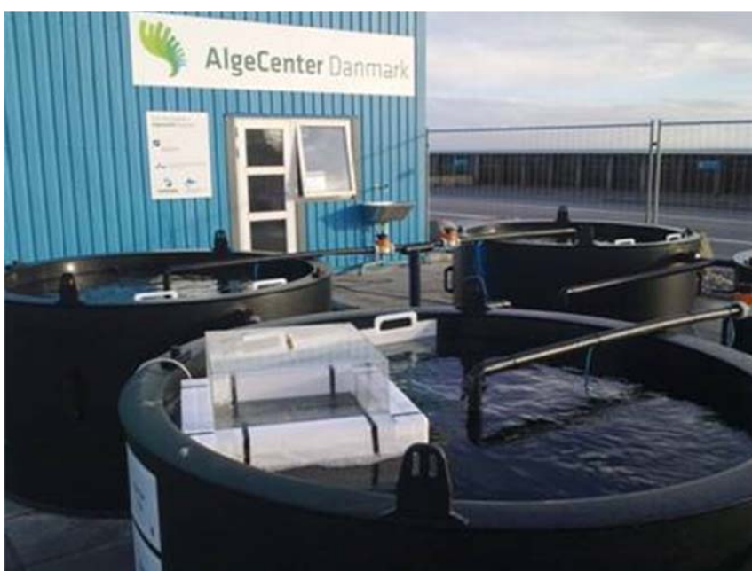
Fig. 2.11 Deployment of floating gas flux chamber to pilot-scale growth basin at the test facility at “AlgeCenter Danmark”, October 2010, Grenaa
