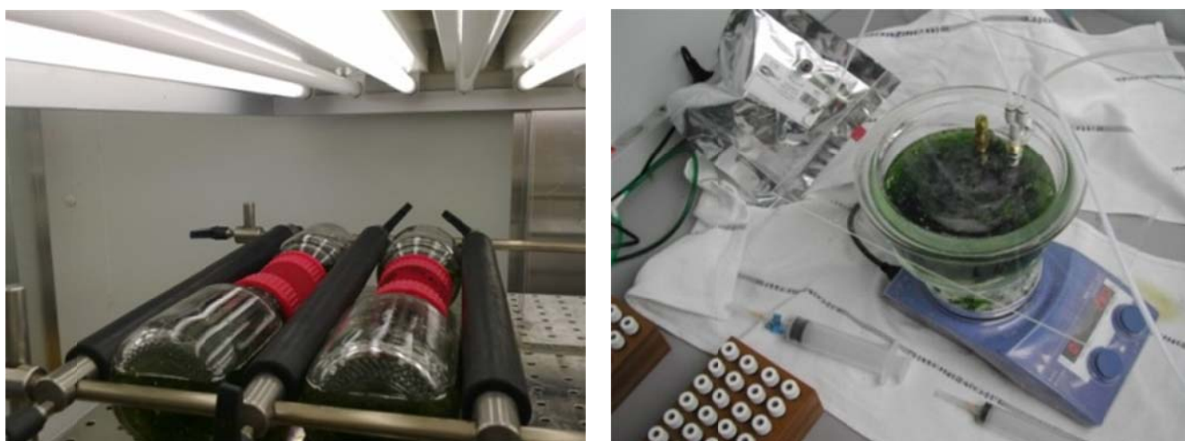
Fig. 2.10 Experimental setup for laboratory incubations of capped static bottles (left hand picture) and flow-through incubator (right hand panel). The laboratory incubations were conducted with different combinations of media, presence of Ulva lactuca biomass and light.
