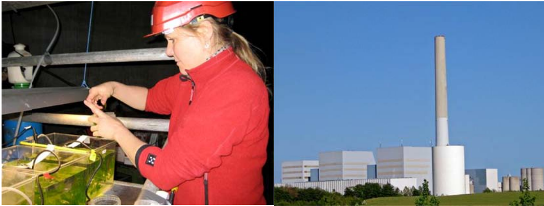
Figure 2.8.a Experiments with cultivation of Ulva lactuca on real flue gas were carried out on-site, inside the chimney at the Studstrup power plant. 2.8.b The Studstrup power plant
