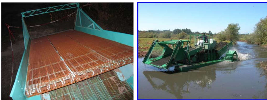
Fig. 4.1 Harvest boat at Zürich See (left) and mechanical harvester from CleanLake Inc. in the USA (right) for bioremediation.
