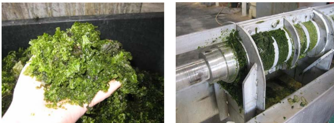
Fig. 4.3 Auger press and Ulva lactuca after pressing but before drying
