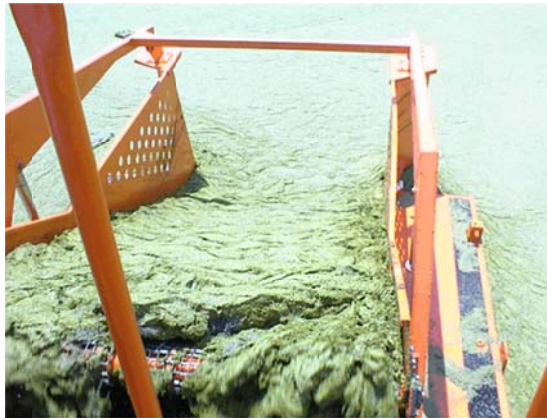
Fig. 5.2 Example of harvesting with conveyor band
