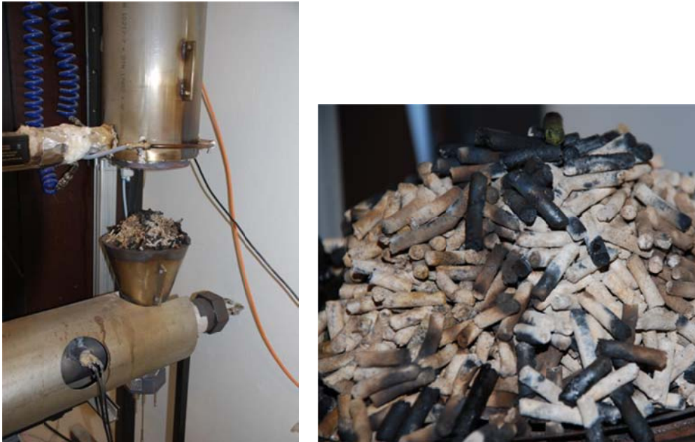
Fig. 4.8 Combustion and ash melting test of Ulva lactuca pellets in The Slagging Analyser was not successful. The very hard pellet could not ignite and the test was stopped. The same situation is experienced with very hard pellets from shea waste.
