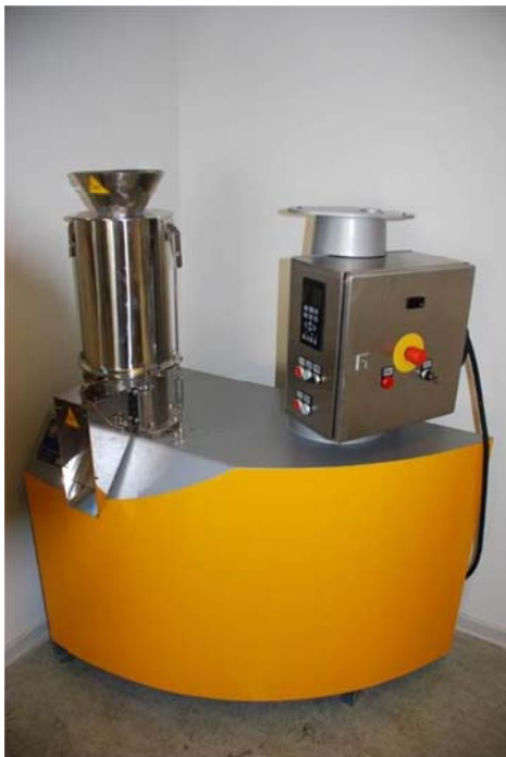
Fig. 4.11 Production of Ulva lactuca pellets on Amandus KAHL pellet press at Danish Technological Institute.
