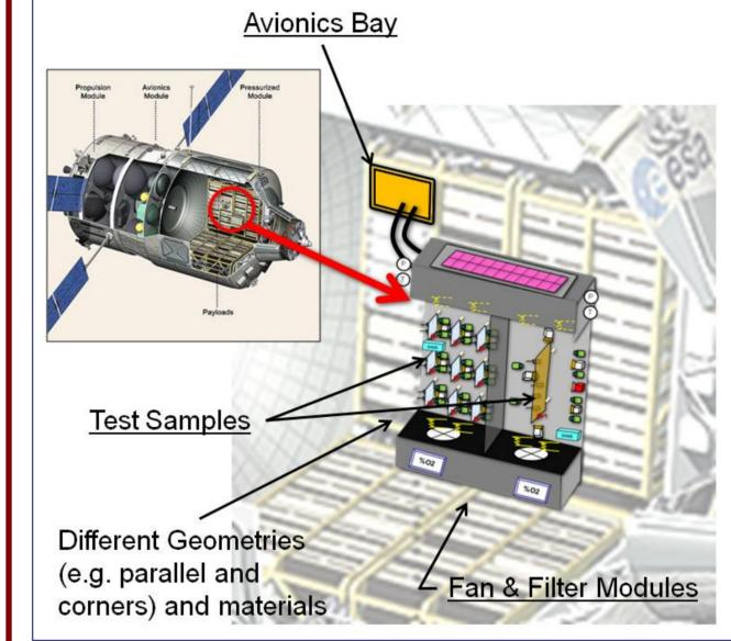
Fire Detection Sensors -Gaseous -Particulate Experiment Equipment:
