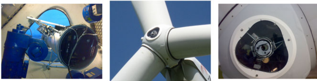
Figure 2. (Left) The upwind scanning spinner lidar installed on the turbine axis in the spinner tip of a 2.3 MW NM80 test turbine, in between the turbines three (blue) pitch-control motors. (Middle) The spinner lidar measures the upwind approaching wind conditions by conical scanning the upwind inflow with a focused laser beam through a hole in the spinner-tip window. (Right) A close-up of the spinner lidar from outside.
