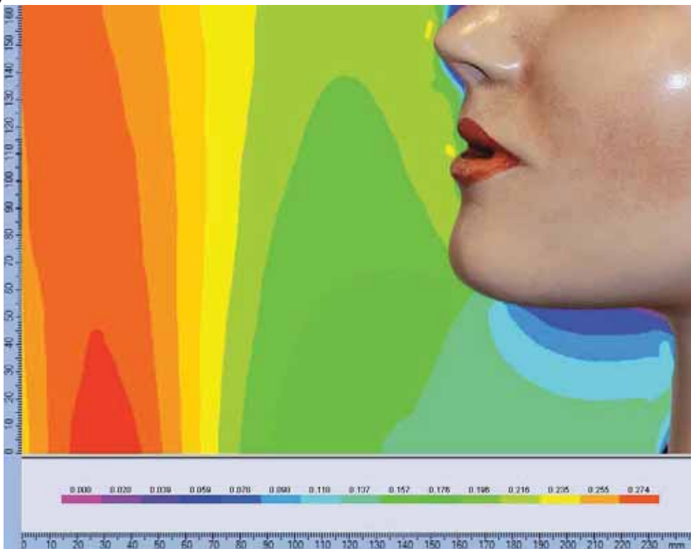
Figure 33 a) Velocity vector diagram showing air direction and b) Contour velocity plot diagram close to the breathing zone of a thermal manikin when heated and box with integrated confluent jets when inner jet supplies 4L/s and outer jet supplies 8L/s.
