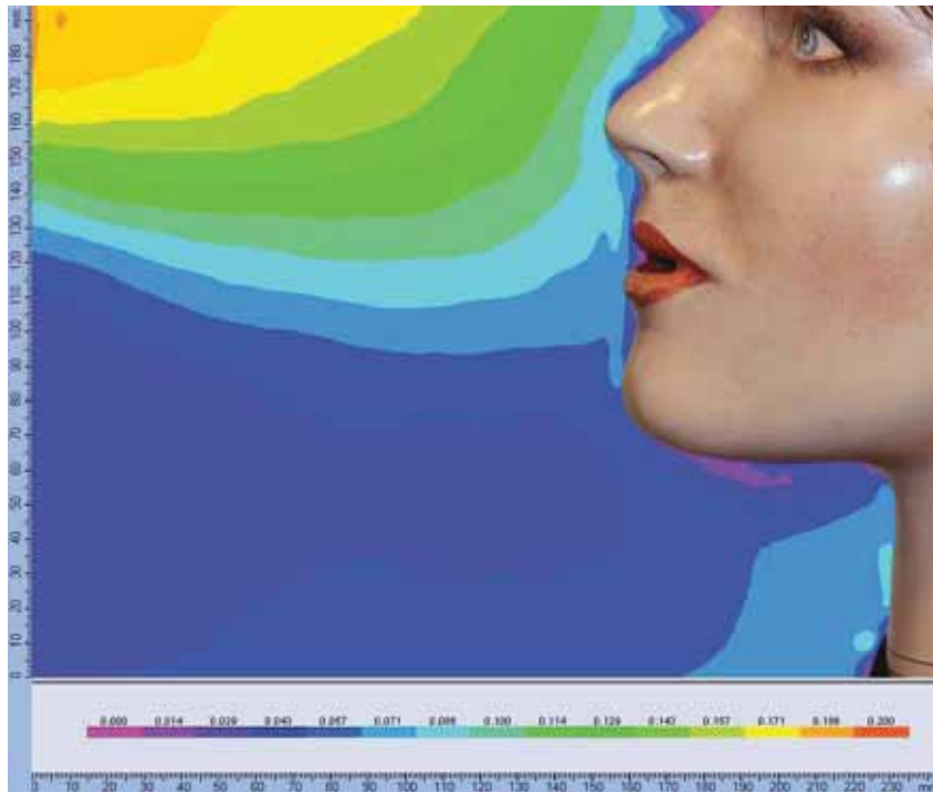
Figure 14 a) Velocity vector diagram showing air direction and b) Contour velocity plot diagram close to the breathing zone of a thermal manikin when heated, with straight board (passive control method) pressed at stomach level and the RMP supplying 4L/s at 0.4m frontally slightly from above.
