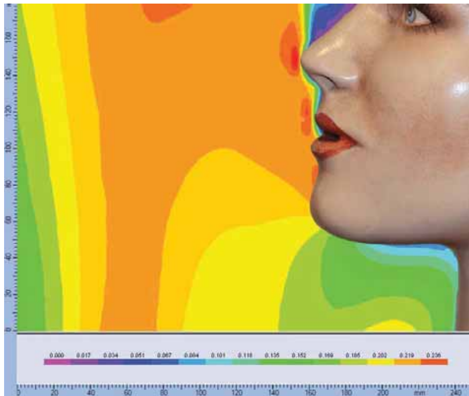
Figure 28 a) Velocity vector diagram showing air direction and b) Contour velocity plot diagram close to the breathing zone of a thermal manikin when heated and box with integrated confluent jets when both inner and outer supply 6L/s.
