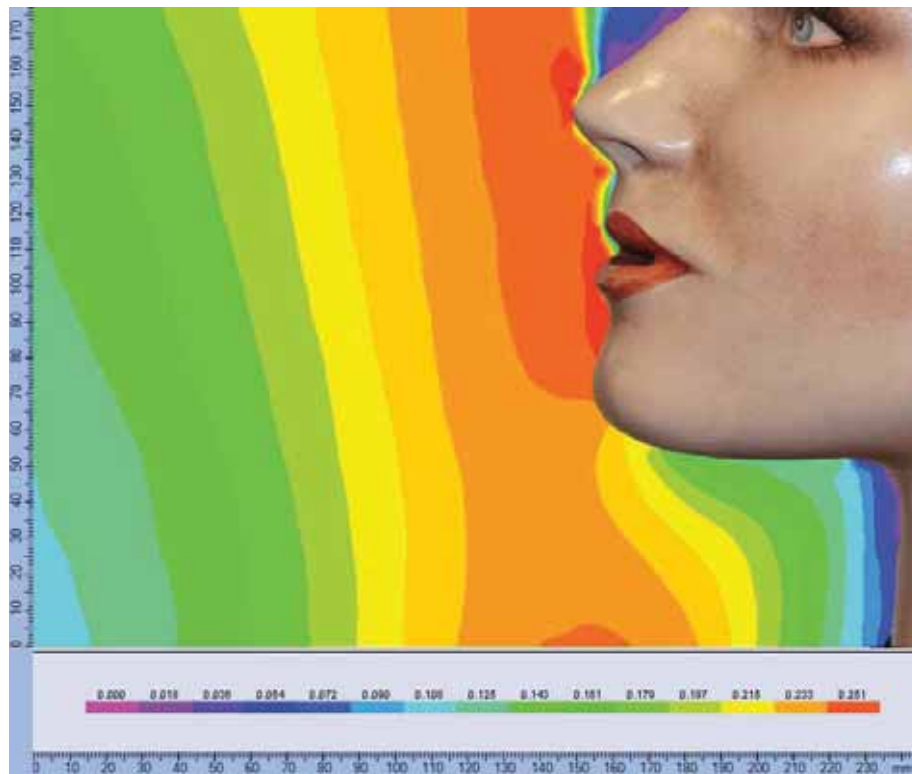
Figure 34 a) Velocity vector diagram showing air direction and b) Contour velocity plot diagram close to the breathing zone of a thermal manikin when heated and box with integrated confluent jets when inner jet supplies 8L/s and outer jet supplies 4L/s.
