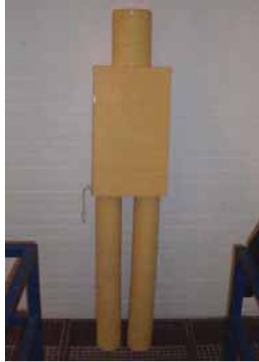
Figure 5.10 Picture of the heated dummy of simplified geometry resembling a human and used to mimic the lying patients in the hospital mock-up environment.
