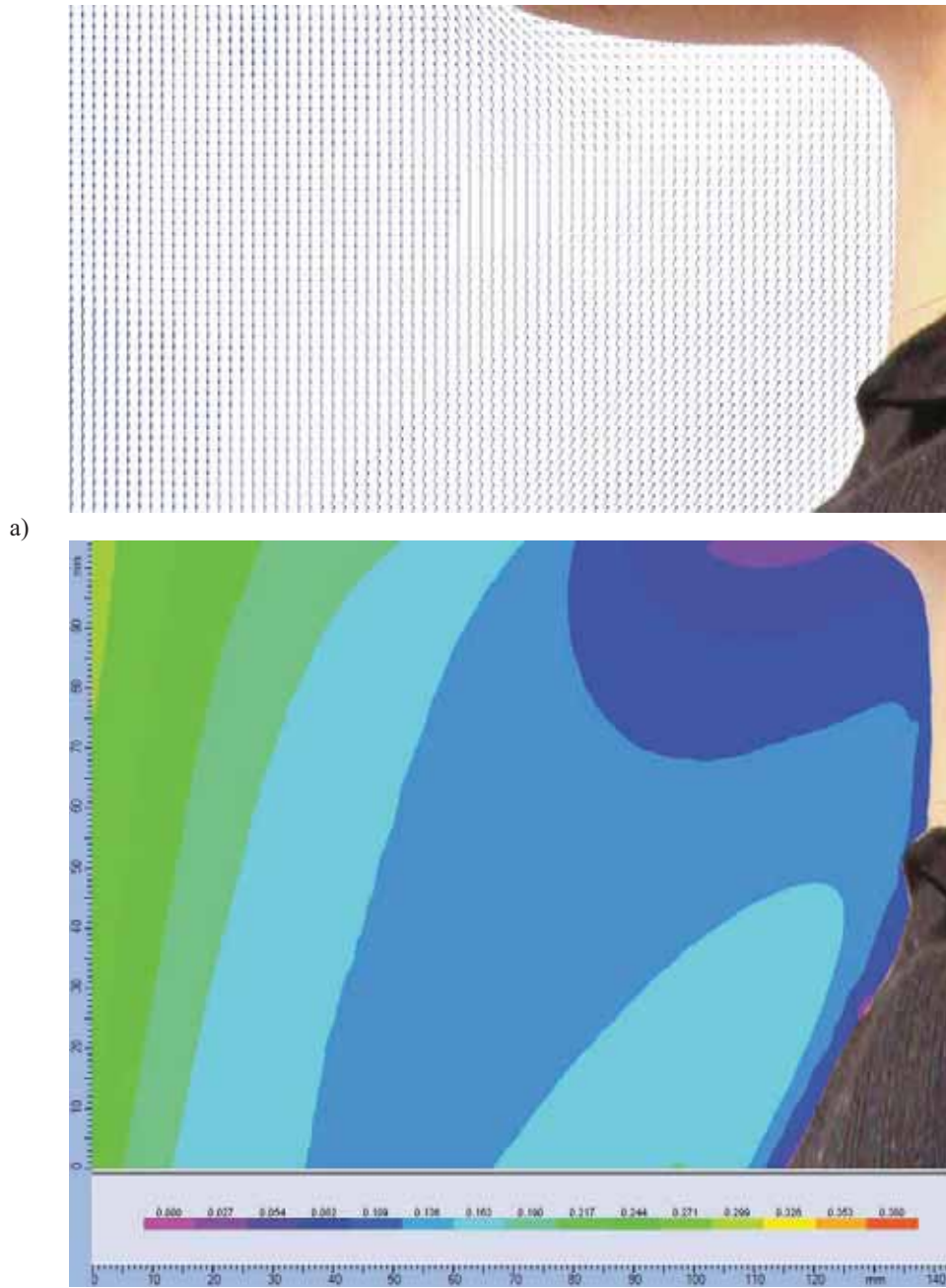
b) Figure 48 a) Velocity vector diagram showing air direction and b) Contour velocity plot diagram close to the heated manikin (neck) and box with integrated confluent jets when inner jet supplies 4 L/s and outer jet 8L/s.
