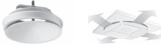
Figure 5.3: Investigated non-motorized diffusers. Left figure: Circular air diffuser with fixed opening area. Right figure: Active diffuser with self adjusting inlet vanes that changes the outlet area depending on the pressure upstream of the diffuser
