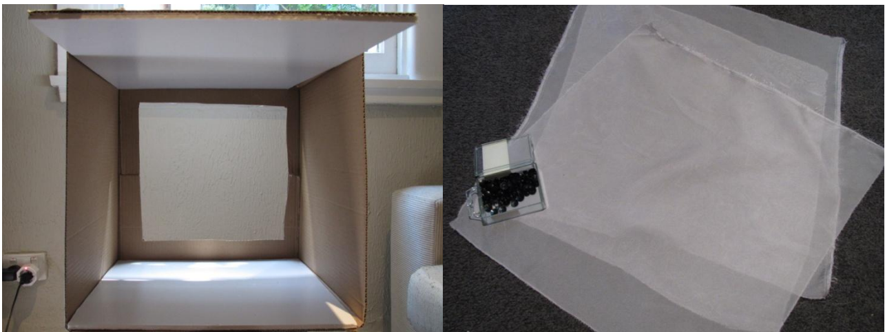
Figure 17 Left: Open ended box with foam board in ceiling and on the floor. Right: Pins and three pieces of fabric no. 1 (polyester chiffon).
