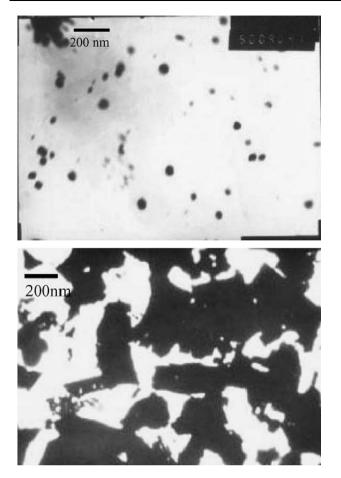
Figure 3 TEM images of  $CeO_2/ZnO$  nanocatalyst prepared by the combining method (top) and ordinary catalysts prepared by the conventional impregnation (bottom).
