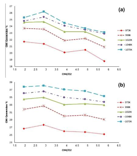
Figure 2 Profile of percent of methane conversion versus  $CH_4/O_2$  over Li/MgO at different feed temperatures: (a) ordinary catalyst, (b) nanocatalyst.
