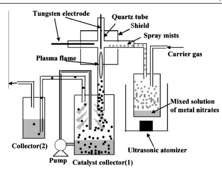
Figure 1 Solution-spraying plasma system for the preparation of nano sized catalysts on hollow oxide balls.
