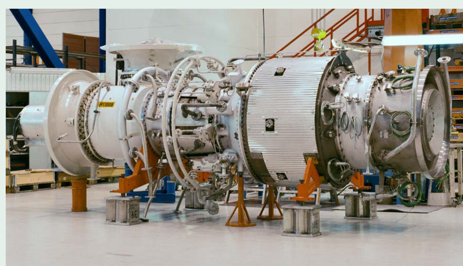
Figure 3: Twin-spool gas turbine Siemens SGT-500
