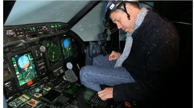
Figure 2: Experiments in baseline physical simulator, with head-mounted eye-tracking equipment
