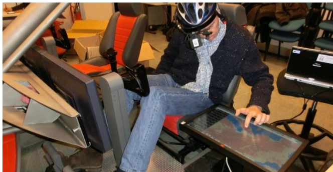
Figure 5: Experiments using the tactile prototype in the low position, and eye-tracking equipment
