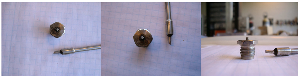
Figure 2.17: Broken Valve Pin
