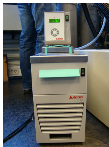
Figure 2.27: Julabo F12 used to Pump Cooling Water Around the System
