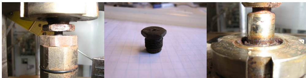
Figure 2.14: Corrosion around the Valve Pin
