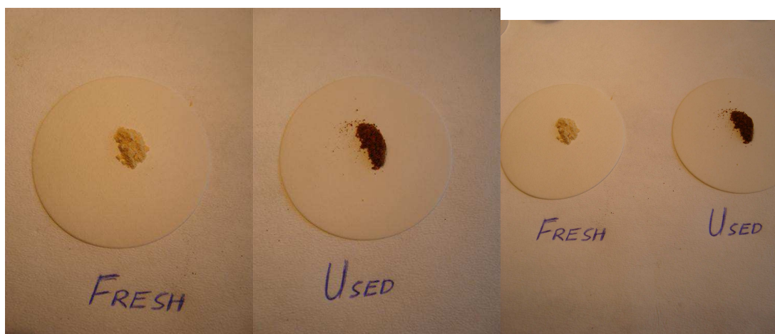
2.5 wt% [\text{Rh}(\text{CO})_2\text{Cl}]_2 with 30 vol% Bmim OH
