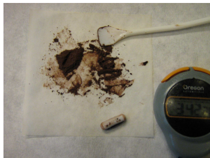
Figure 4.6: Discoloured SILP in Air
