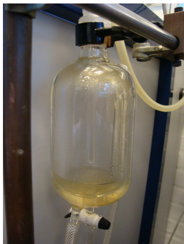
Figure 2.30: Condenser Containing Condensate from System
