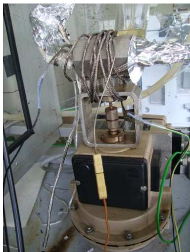
Figure 2.18: Heating Cable used for Pressure Valve
