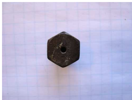
Figure 2.16: Surface of the Pin Seat Showing Black/Brown Condensate
