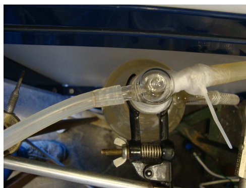
Figure 2.31: Condenser from Above, Showing Inlet and Outlet to Condenser
