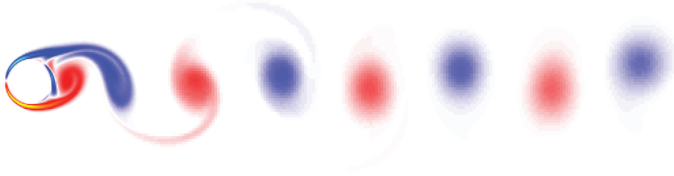
Figure 1.2: The von Kármán vortex street behind a circular cylinder at Re=500 . Visualisation of vic20 simulation.
