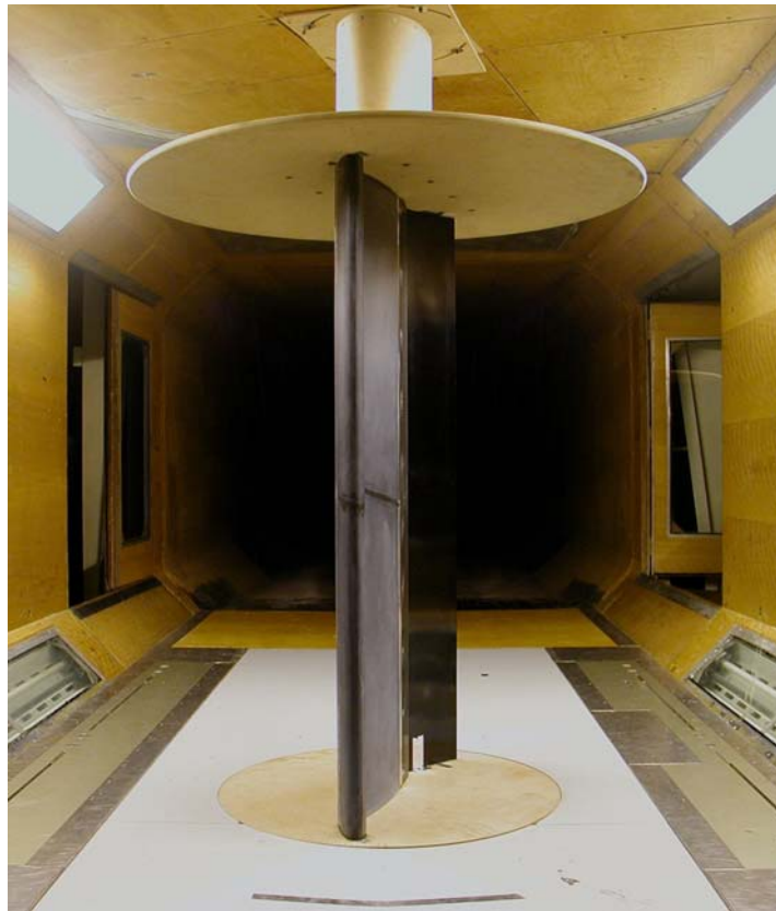
Figure 12: High-lift model mounted vertically in 8'×6' wind-tunnel
