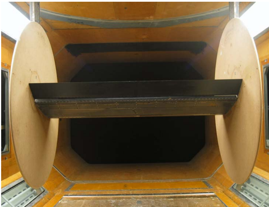
Figure 13: High-lift model mounted horizontally in 8'×6' wind-tunnel
