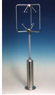
Figure 5.2.1: The sonic anemometer Solent R3 from Gill. The three acoustic paths has a length of 149 mm.
