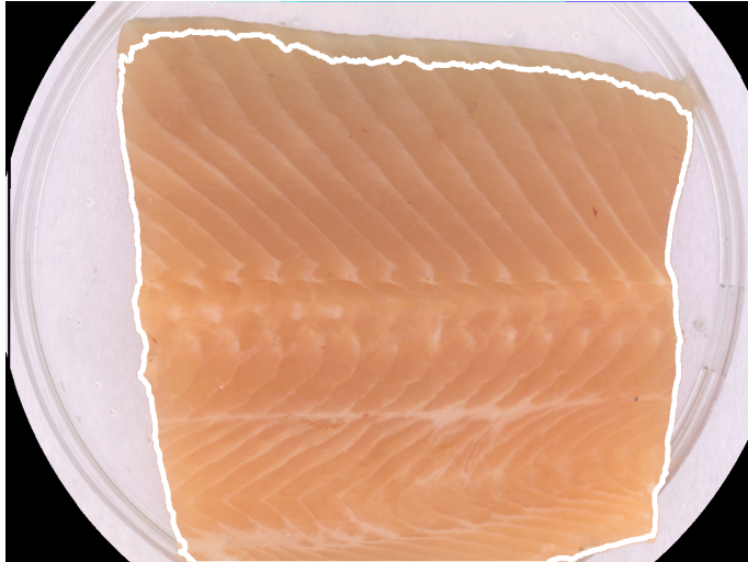
Figure 11: Trout fillet image example. An sRGB representation of the multi-spectral VideometerLab image, with the segmented ROI visualised with a white outline.
