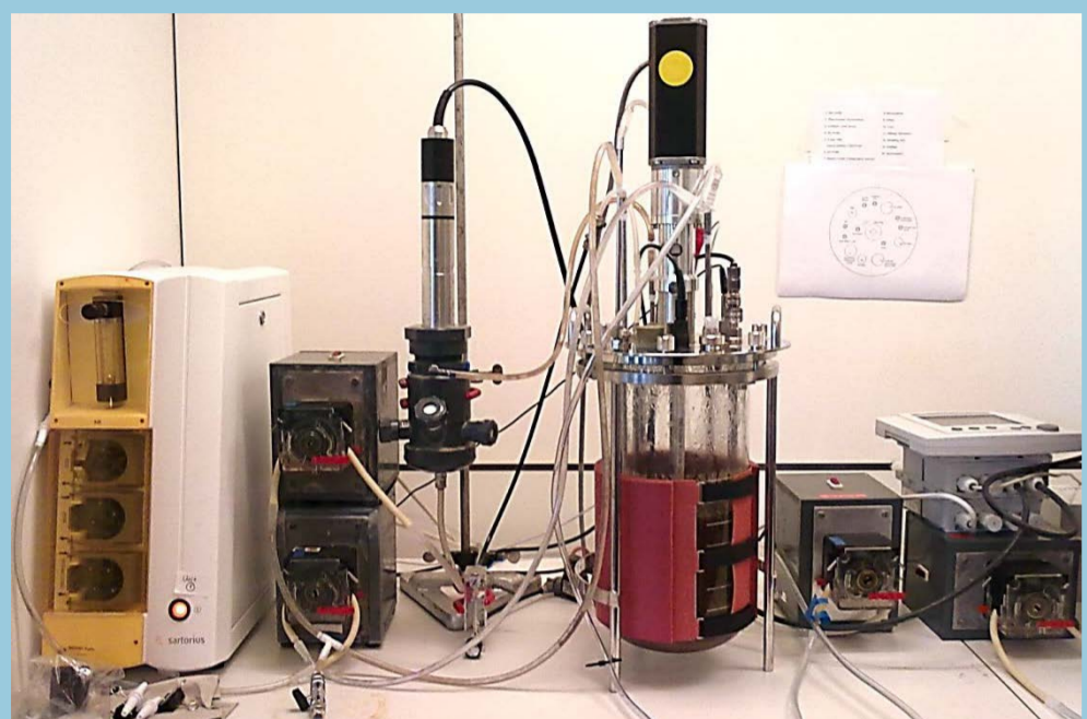
Lab-scale (4L) sequencing batch reactor (SBR) performing single-stage nitritation/anammox with intermittent aeration
