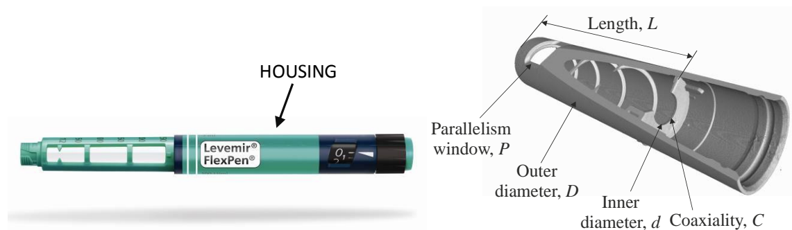
Fig. 2. (a) Insulin pen; (b) Definition of measurands
