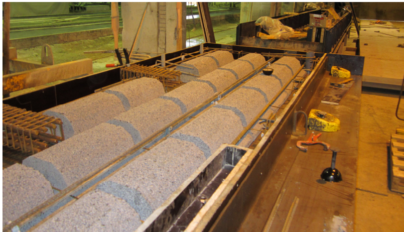
Fig. 2 – Production of a super-light slab element.
