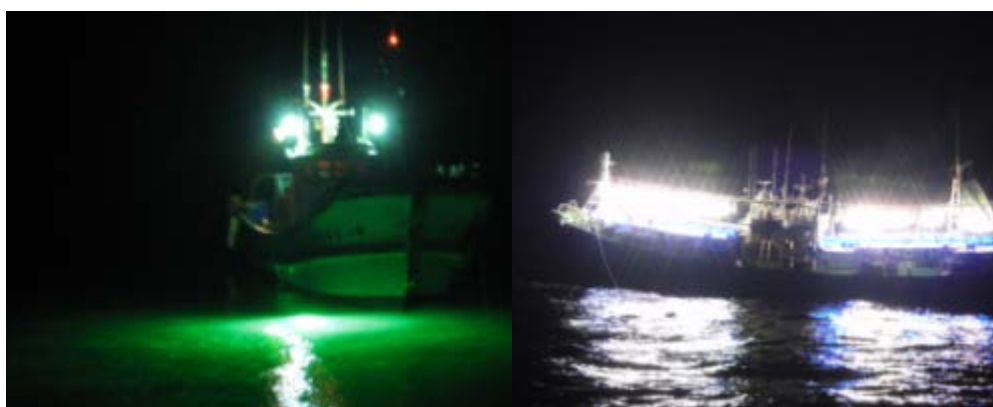
Figure 11. Squid jigging (left; only surface light) and purse-seine boats (right; surface and underwater lights).
