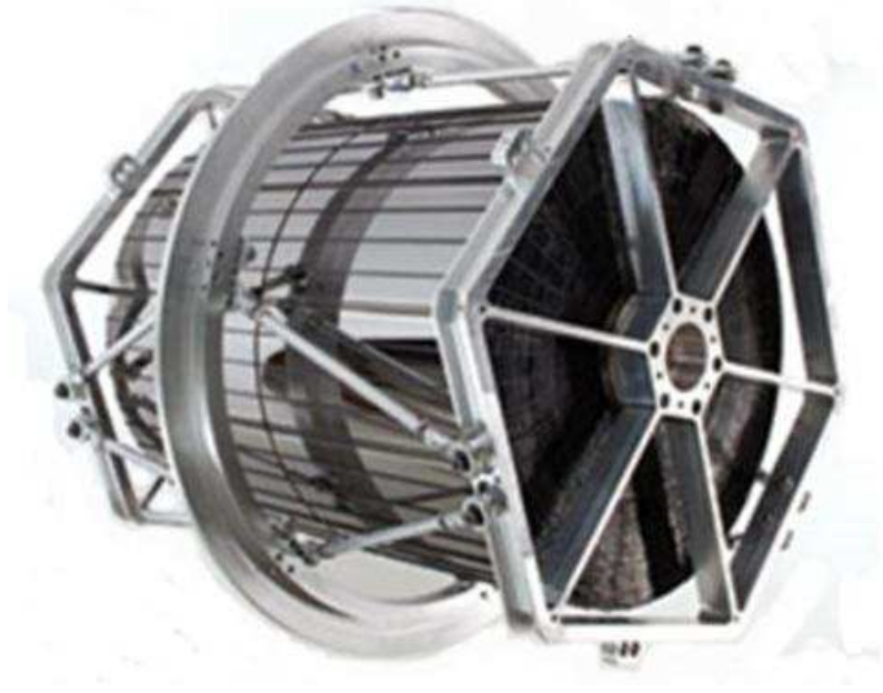
Figure 1.10: Photo of FM1 mounted in its calibration fixture. Photo credit: Scientific American.
