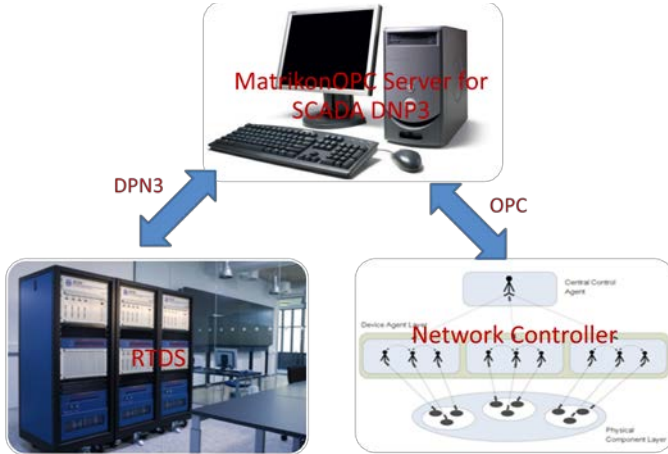
Figure 2 Simulation platform for active distribution network controller
