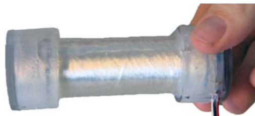
Figure 2. Cylindrical DEAP actuator
