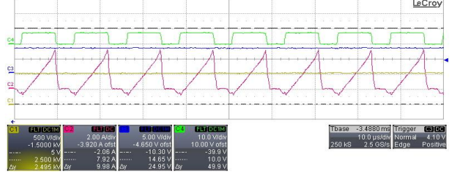
Figure 15. Experimental waveforms (CH1-Output voltage; CH2-Primary current; CH3-Charge signal to the converter; CH4-Mosfet gate voltage)
