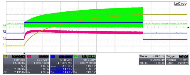
Figure 14. Experimental waveforms (CH1-Output voltage; CH2-Input current; CH3-Charge signal to the converter; CH4-Mosfet drain voltage)
