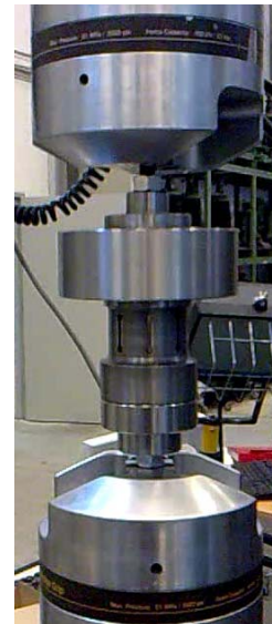
Figure 7: Axial Sliding Test mounted on a tensile machine.
