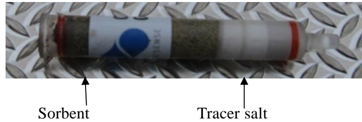
Figure 12: The flow-through passive sampler, SorbiCell.
