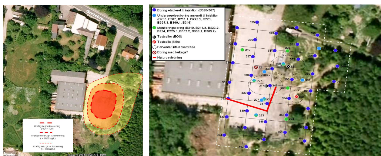
FIGURE 1. Sortebrovej site. TCE-contamination and network of injection wells for substrate and bioaugmentation culture injection in clay till.
